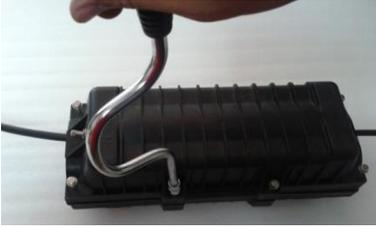
Be careful for side - gasket not to protrude out of groove or fold , put the upper case on the lower case and then tighten all bolts in diagonal order.
