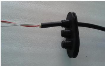
Pass the fibers through protection tube and make protection tube overlap 0.8"(2cm) of loose tube and passing the cable through end-gasket as on the picture left.
