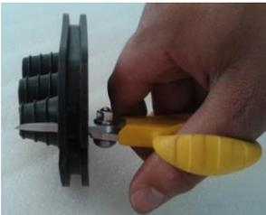
cut the port of end-gasket by exterior diameter of each cable before cutting a edge of end-gasket at the angle of 45 degree , making the cross section plain.
