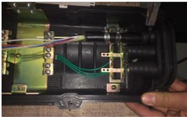
clamp the cable on the bracket with hose clamp .Before covering upper case ,tighten the hose clamp with a screw once again.
