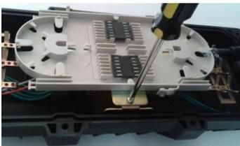
Place a tray on the bracket and then fix it with bolts.
