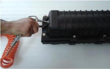
Inject air into closure in 6psi or less pressure and smear soapy water around the closure - connection line and see if sealing is secured.
