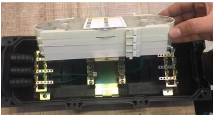
Unscrew the bolt on the bracket inside the closure and flip over the tray.
