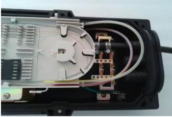
After splicing , apply splice - sleeves to the point of splicing and place them for each lane on the tray and then arrange the rest bundle of fiber in the tray.
